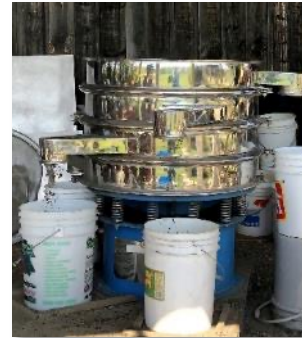
MATERIAL SEPARATED INTO DIFFERENT SIZE FRACTIONS
